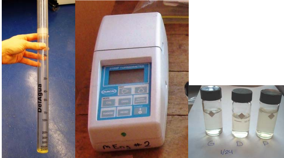
Figure 31 Turbidity tube (left), Hach® turbidimeter (center), and Hach® turbidity vials (right)
