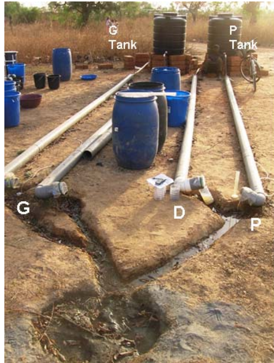
Figure 55 Pilot HRF Ghanasco Dam, Tamale, Ghana Photo Credit: Carl Allen
