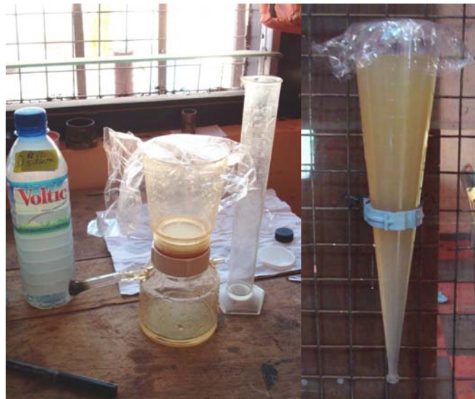
Figure 32 Filter setup (left), Imhoff Cone (right)
