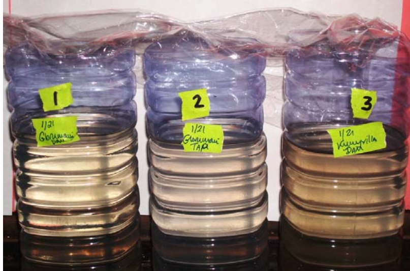
Figure 33 Settling stability test on dam water at the TSO (January 21, 2008)
